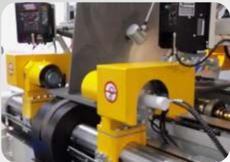
INLINE FLANGE STRAIGHTENING
