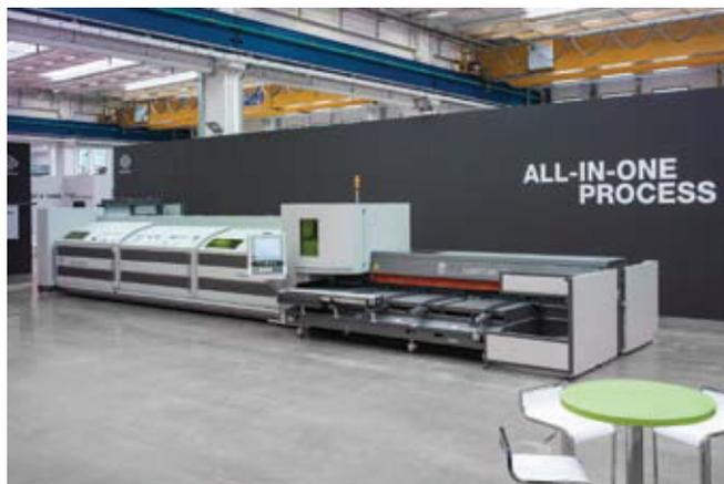
**The “All-In-One” process demonstrated one Lasertube machine for cutting straight tubes, one tube bending machine and a 5 axis laser cutting machine with a handling robot**
