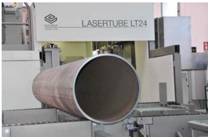
**The new LT24 equipped with a 3.5kW CO2 laser extends the laser tube cutting capability to 24” diameter i.e. from actual 508mm to 604mm diameter tubes**
