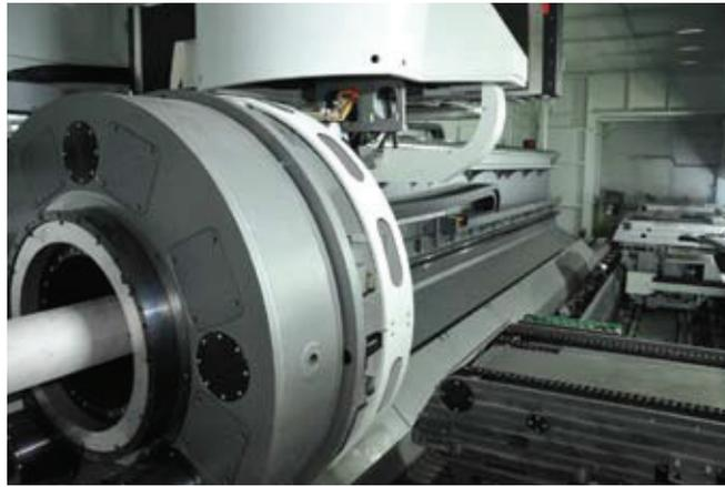
**Adige-Sys presented major innovations, like the new LT14 fiber. This machine belongs to the Jumbo series and was equipped with a 3 kW fiber laser source and the new 3D TubeCutter head for the first time**
